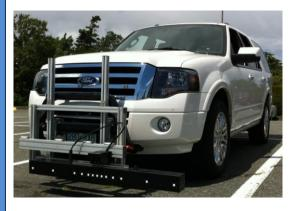
The SMF/M is a world class system for the photometric measurement of Airfield Ground Lighting system according to ICAO Annex 14 recommendations.
